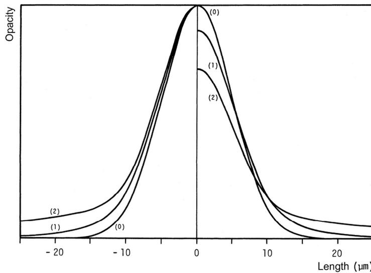
Fig. 3 : Spread function according to formulas (0), (1) and (2) for a  $\sigma = 14 \mu\text{m}$ . Left diagram : functions without normalization, right diagram : normalized curves. One notices the effect of the contrast reduction of small signals when the base of the spread function is enlarged.
