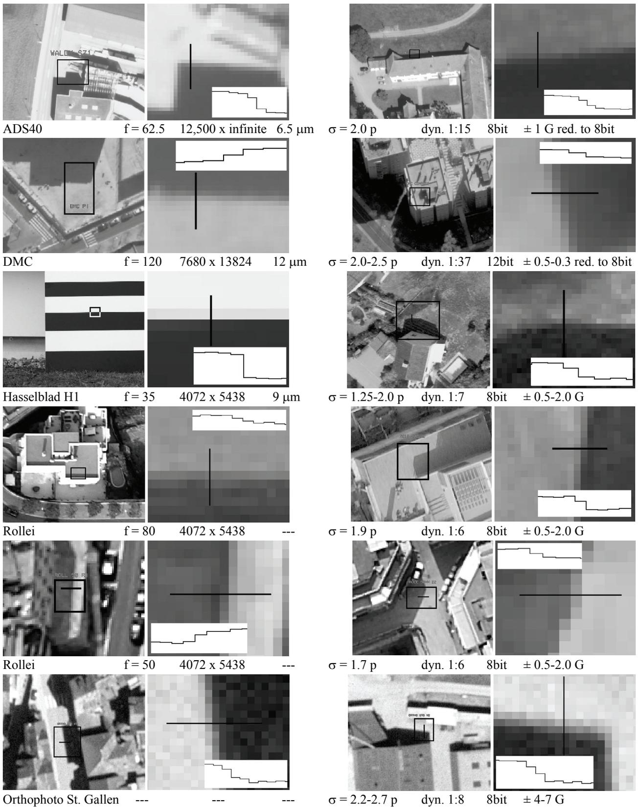
Fig. 6 : Extraction of digital images and micro enlargement with the presentation of the grey value profiles. The images show some differences in the image quality. The numerical values characterize the camera, after the focal length is given the size of the image sensor in pixels, follows the pixel size in microns and the spread of the point spread function. Dyn stands for the dynamic range and the last value gives the image noise.
