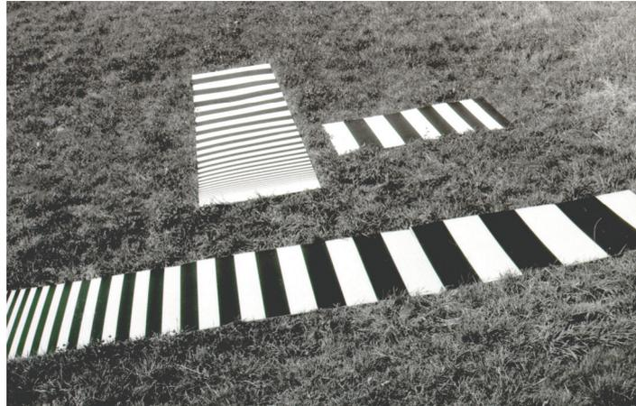
Fig. 5 : Targets for the determination of the modulation transfer function.
