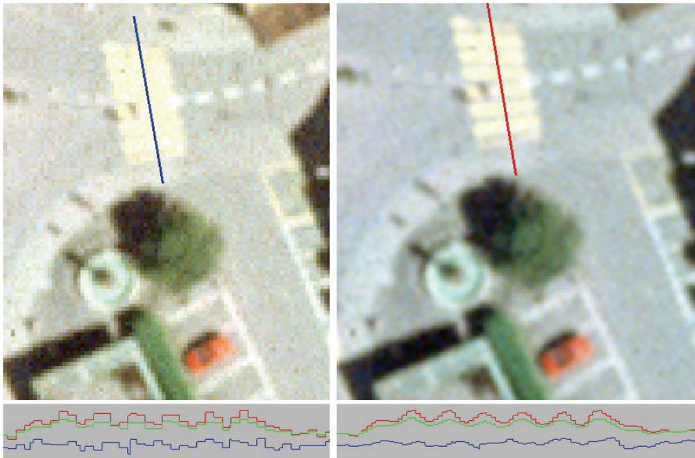
Fig. 1 : Orthophoto GSD 25 cm. Left : original pixel size, right : subsampled to 12 cm. The lower part shows the density profiles over the pedestrian crossing (upper line : red band, lowest line : blue band). Image reproduced by courtesy of the Vermessungsamt St. Gallen.
