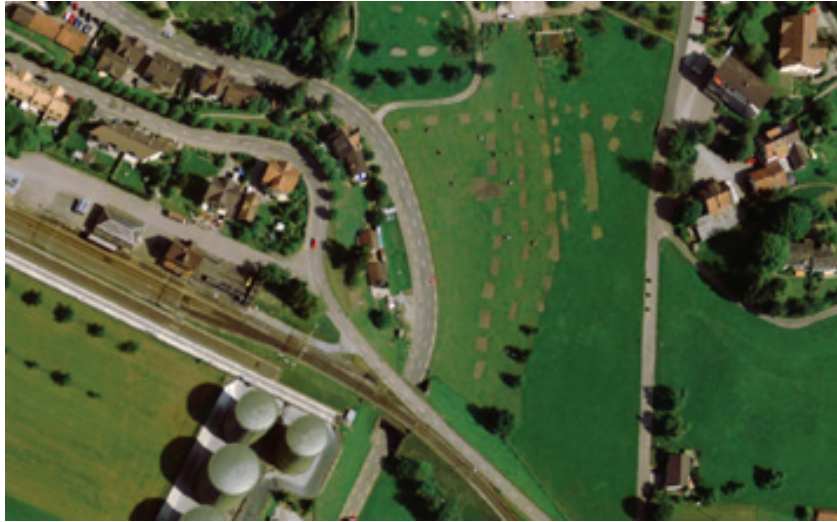
Figure 7: Part of a 10km long, 20cm GSD stereo pixel carpet with constant stereo angle and viewing angle.
