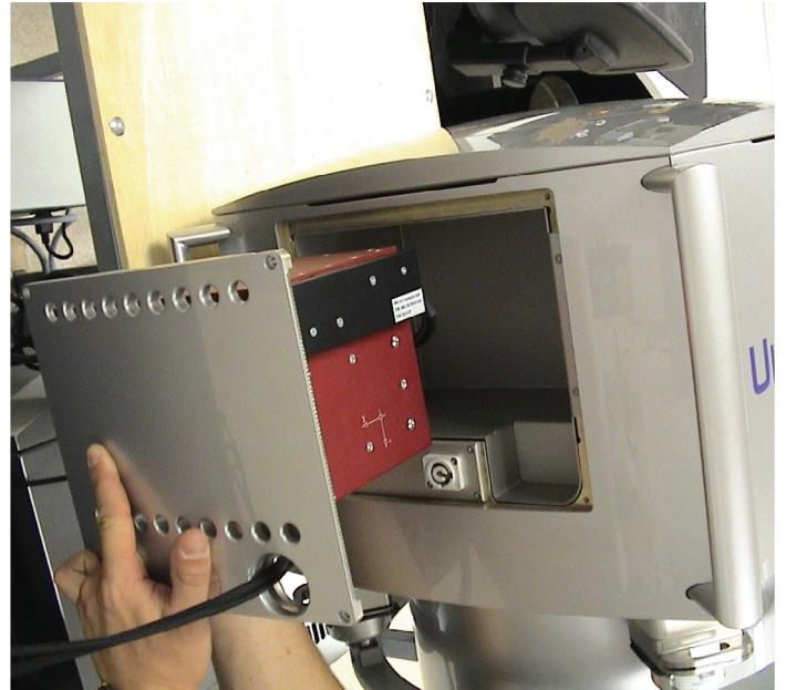
Figure 2: *ULTRACAMD with AEROcontrol IMU ©Z/I Imaging*
