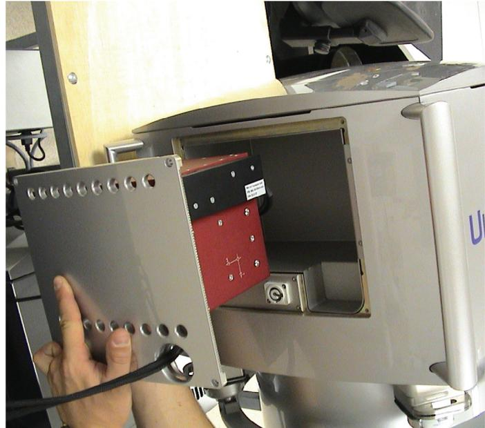
Figure 2: ULTRACAMD with AEROcontrol IMU ©Z/I Imaging
