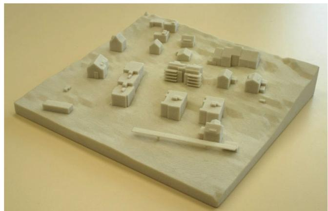
Figure 7: Hardcopy 3D city model of the same area exported from the 3D GIS and produced with a 3D plotter.
