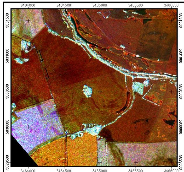
Figure 4: E-SAR false colour composite  $X_{HH}$ ,  $L_{HH}$ ,  $P_{HH}$  (April 2002).
