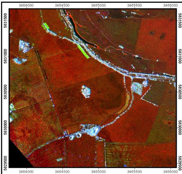
Figure 3: E-SAR false colour composite  $X_{HH}$ ,  $L_{HH}$ ,  $P_{HH}$  (April 2001).
