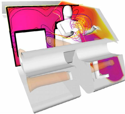
Figure 4: Climate simulation in a car cabin( data courtesy DaimlerChrysler Research): coloured cutting plane, particles paths and isosurface used for visualization
