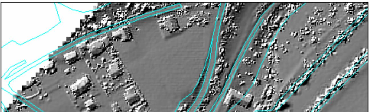
Figure 1: Structure lines acquired by photogrammetric compilation, laid over the DSM derived of laser scanner data.
