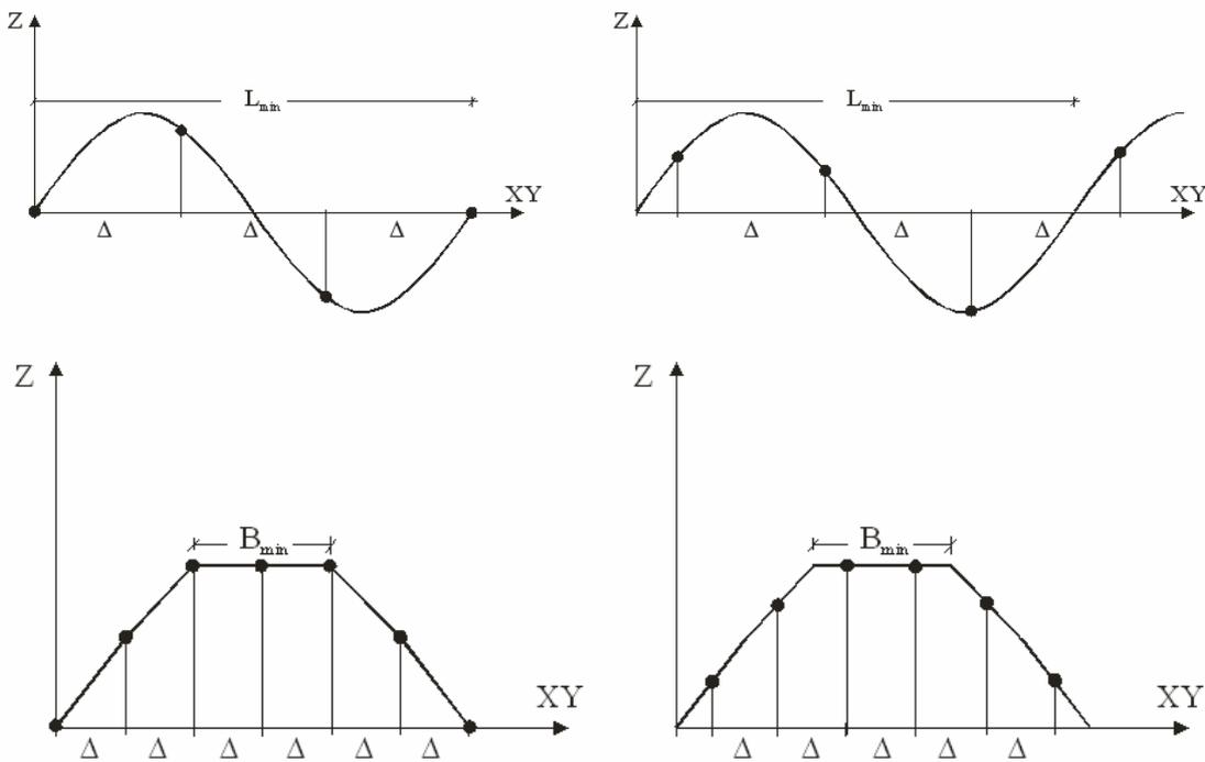
Figure 8: The minimal wave length of a terrain profile (upper sketch), and minimal crown width of a dam in a cross section (lower sketch), in each case with two sets of points from data collection ( $\Delta$  – the point distance).
