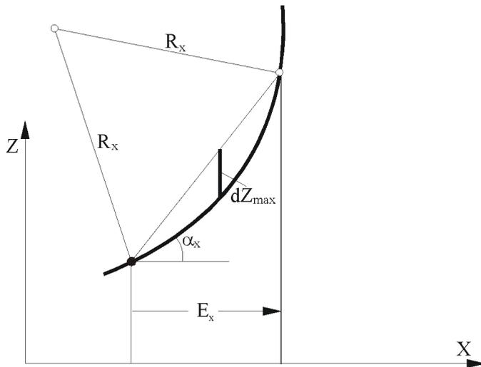
Figure 9: Maximal allowable distance  $E_x$  as defined by the radius of curvature  $R_x$ , by terrain slope  $\tan\alpha_x$ , and the threshold for approximation accuracy  $dZ_{\max}$ .
