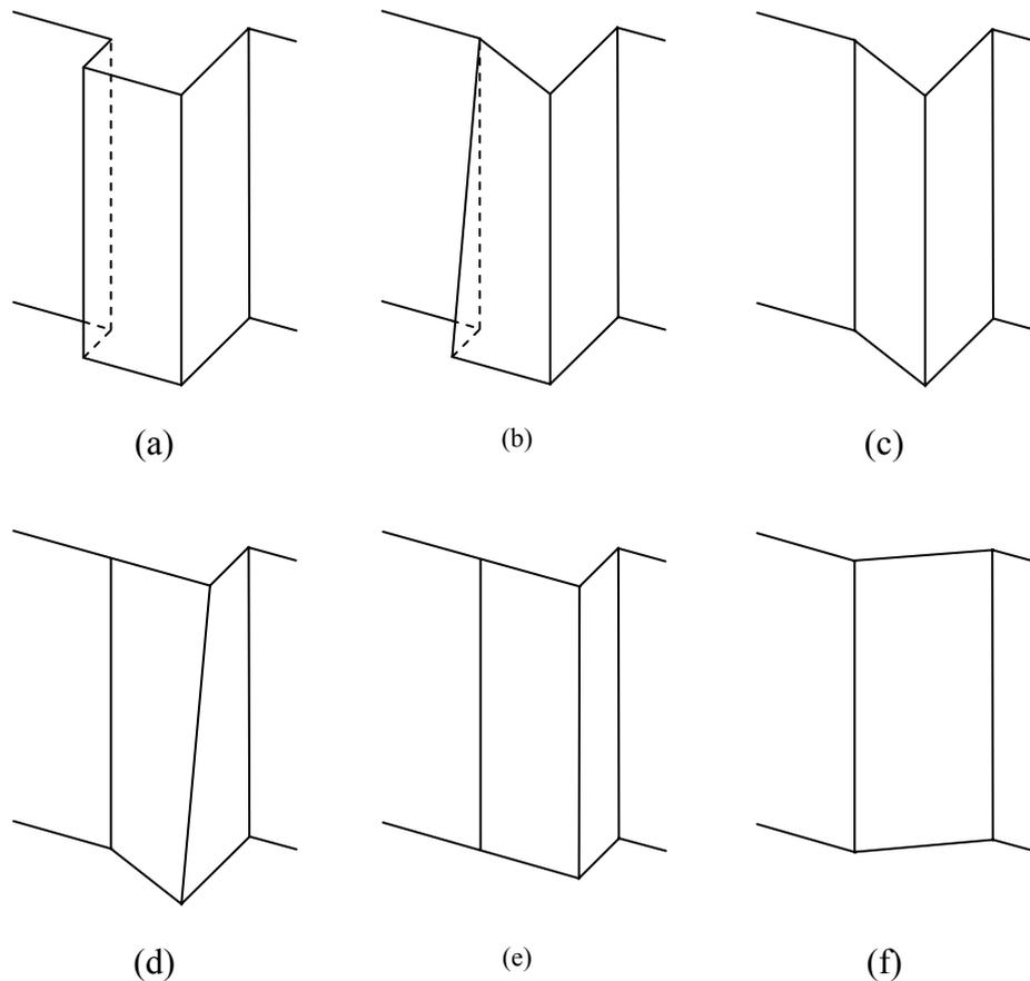
Figure 3: (a-e) Removal of an extrusion: The endpoints of the short edges are collapsed into their base vertices (b+c), whereas the longer edges are foreshortened by the same length (d+e). Collapsing all edges results in the removal of too much geometry (f).
