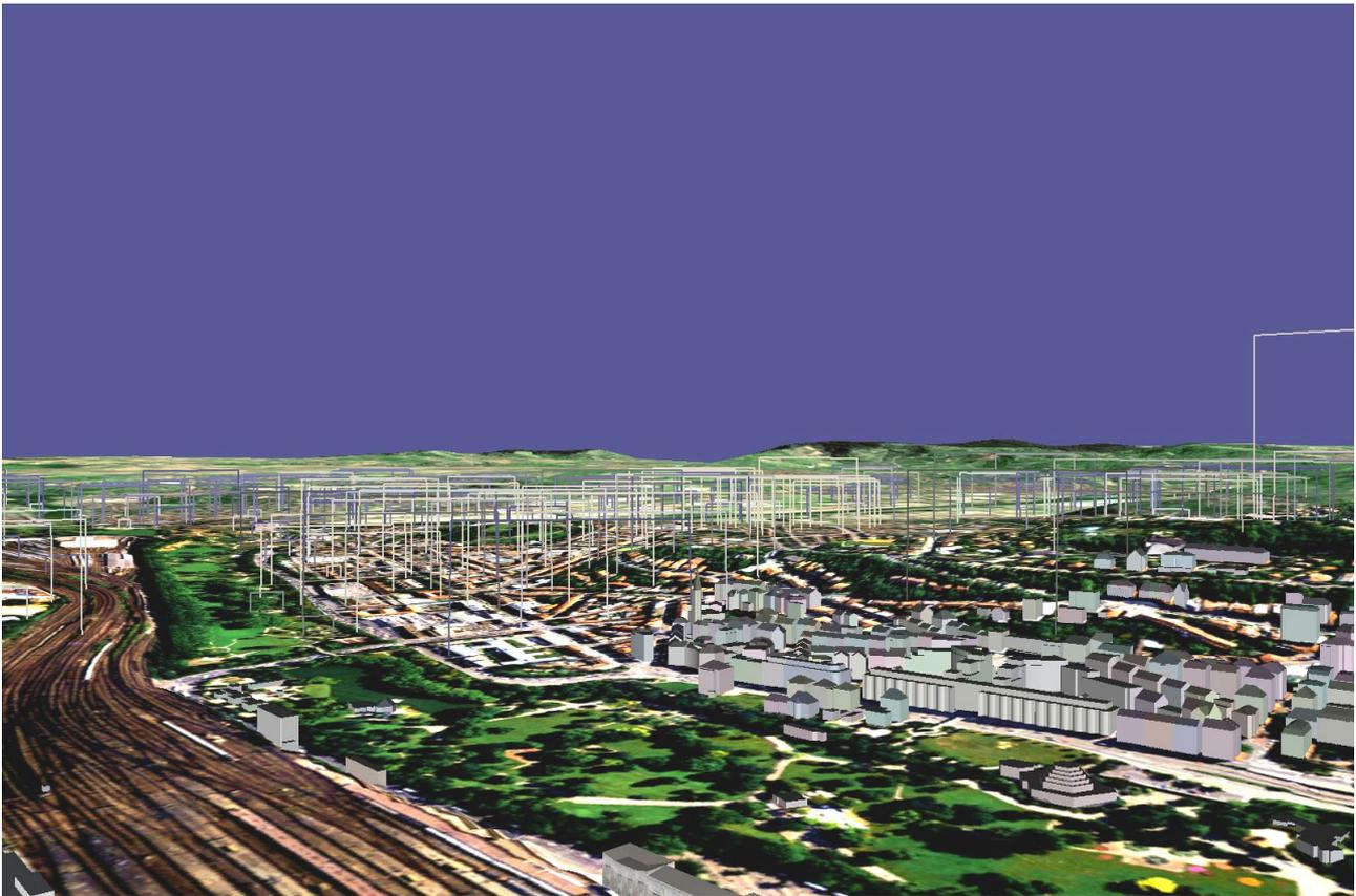
Figure 4: Building objects that are located beyond a distance threshold are rendered as impostors as depicted by the quadrilateral impostor frames.
