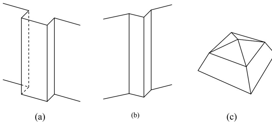
Figure 2: Feature detection distinguishes between faces, edges and vertex-based features: e.g. (a) extrusion, (b) notch and (c) tip.
