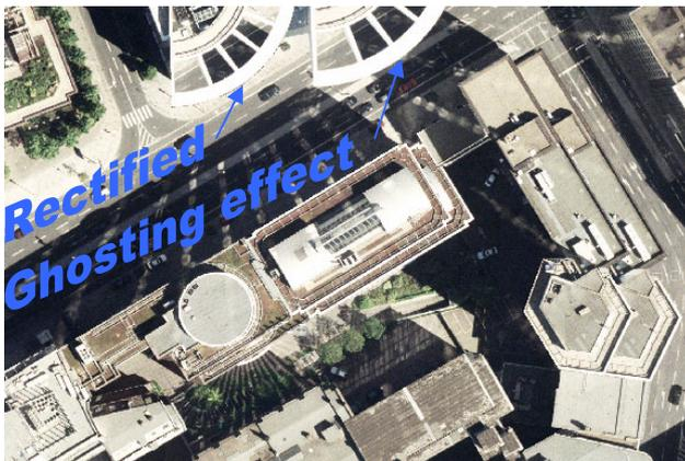
Figure 2 Ghosting effect due to the use of a DSM in a city without detection of occluded areas, even if the building is correctly rectified
