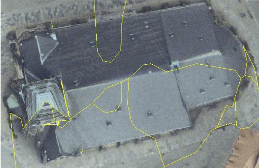
Figure 10 True-Orthophoto mosaic with automatically detected seam lines.
