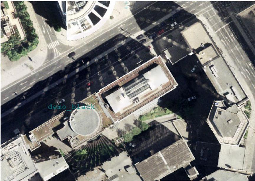
Figure 5 True-Orthophoto produced with OrthoBox. Occlusions automatically replaced by using several overlapping orthophotos.
