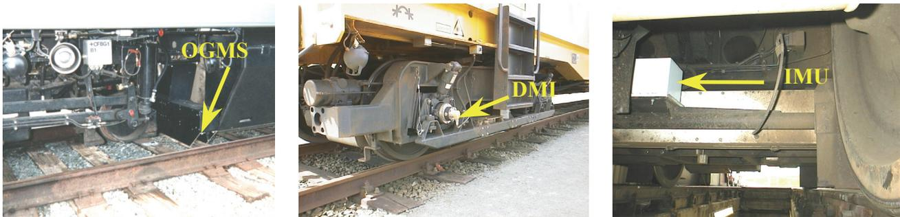
Figure 5 POS/TG hardware installation: OGMS installation (left), DMI Installation (middle), IMU Installation (right)
