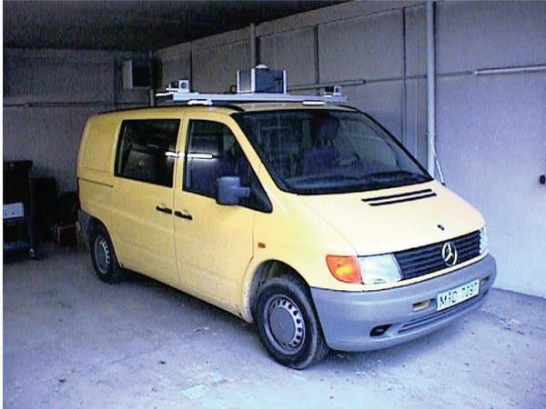
Figure 7 POS/LV installed on a van for mobile mapping
