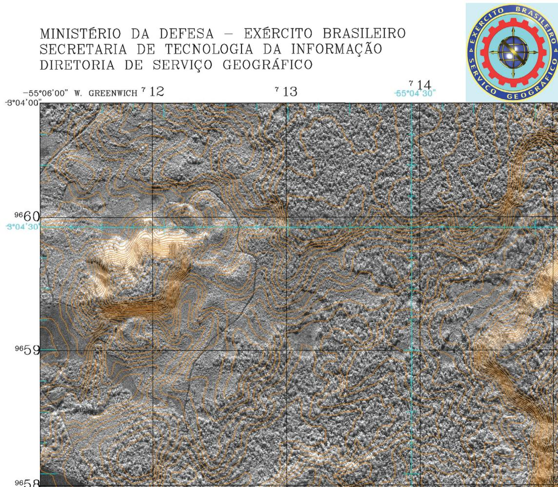
Figure 6: Part of a SAR orthoimage map with DGM contour lines in a scale of 1:25 000 generated from X- and P-band data by DSG, Brazil.
