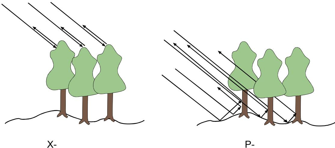
Figure 1: Penetration dependency on radar frequency. Black arrows indicate transmitted and reflected X-band and P-band waves on top of the trees and on the forest floor.
