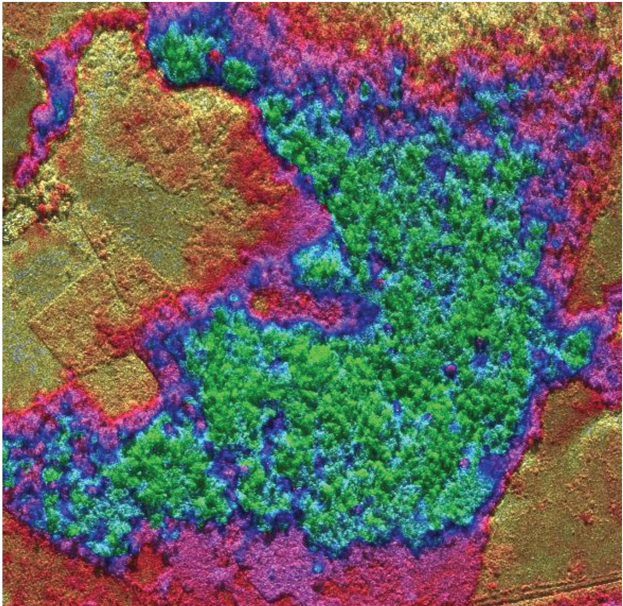
Figure 5: Difference map of DSM and DGM data of an area of approx.  $2 \times 2 \text{ km}^2$  (bright green = 30 m, dark green = 0 m).
