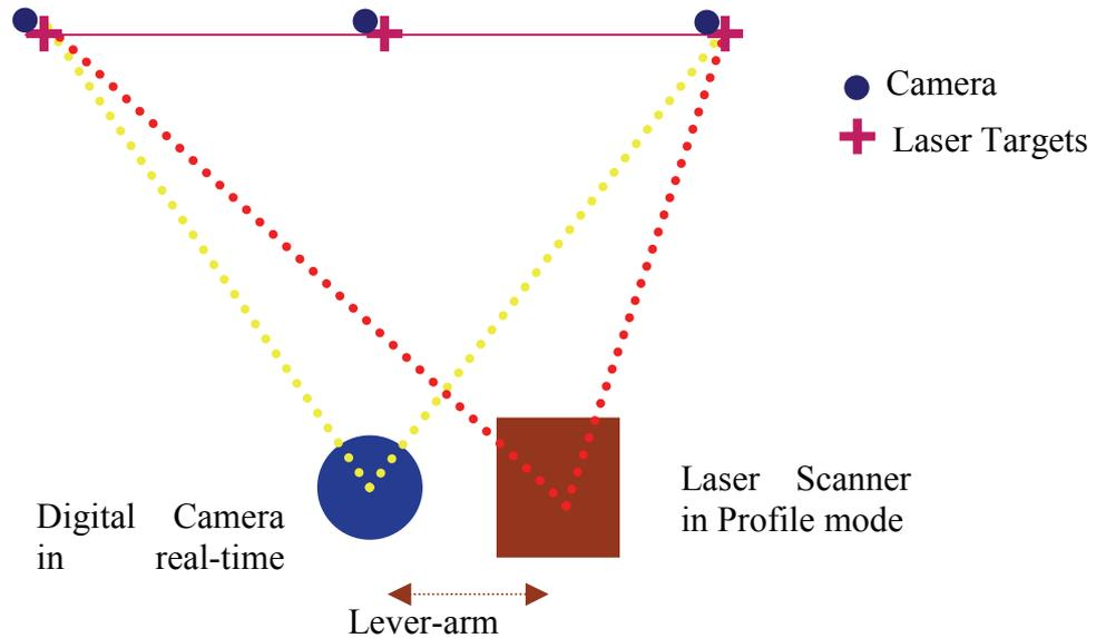
Figure 4: DORIS Camera/Laser Lab Coarse Alignment
