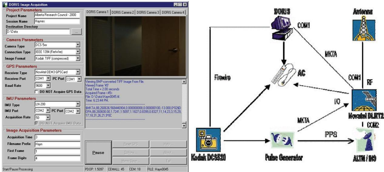
Figure 2: DORIS In-flight Data Acquisition Software and Hardware
