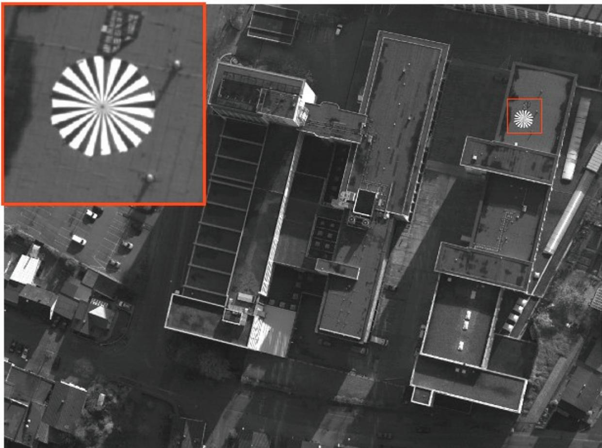
Fig. 11 Detail of figure 10, flying height: 740m above ground, GSD = 3"
