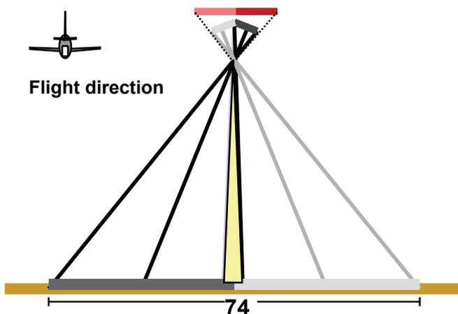
Figure 9. cross track coverage of dual camera head
