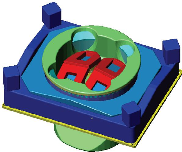
Figure 6. Panchromatic channels in gyro stabilized mount
