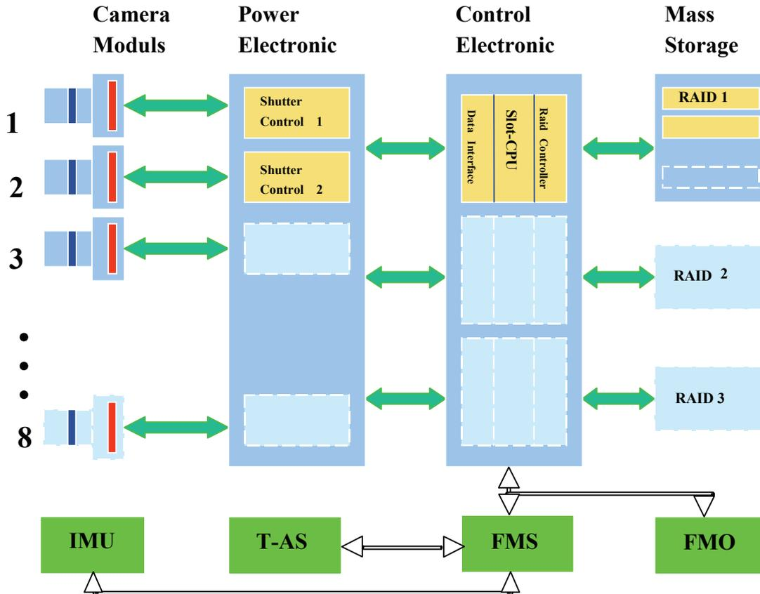
Figure 3. Block diagram DMC flight system
