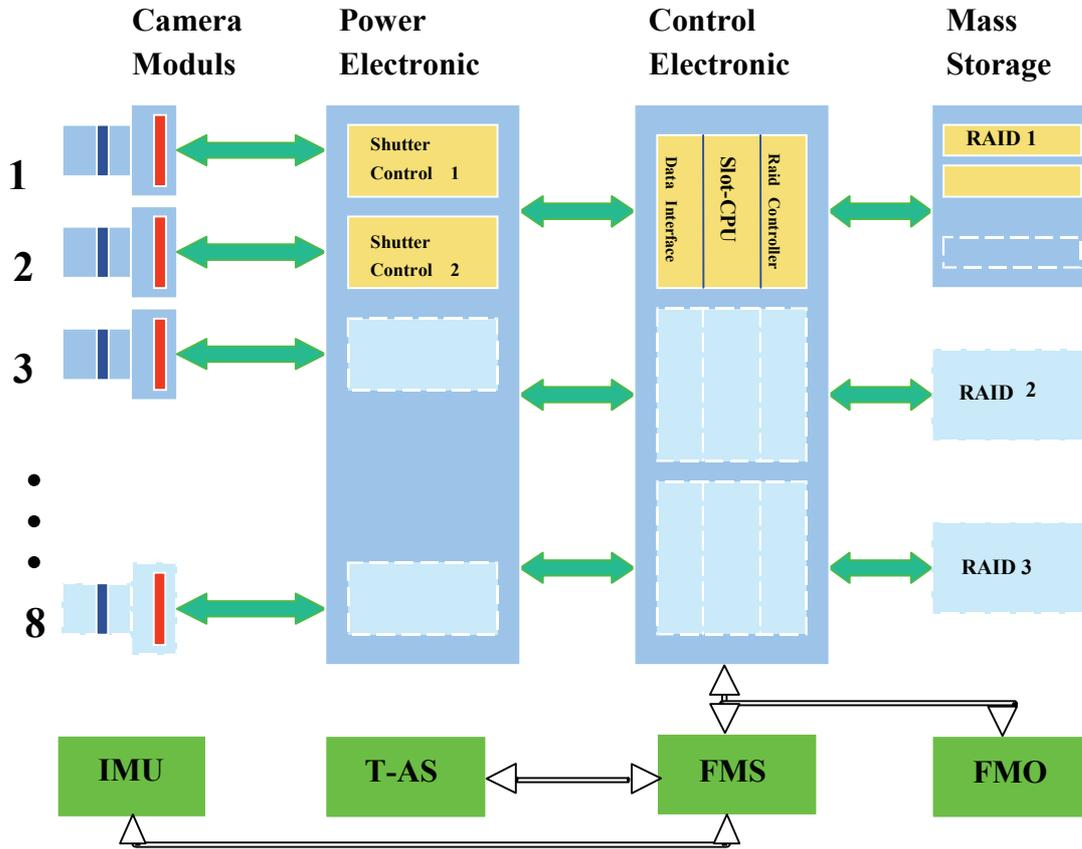
Figure 3. Block diagram DMC flight system
