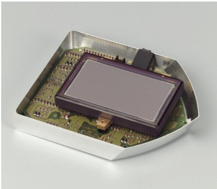
The figure shows the 7k\*4k CCD-Chip and the front end electronics.
