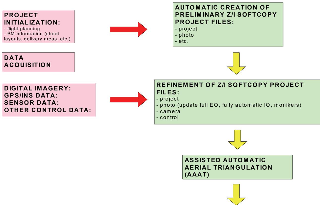
Figure 3: Illustration of the possibilities for a seamless, highly automated production workflow
