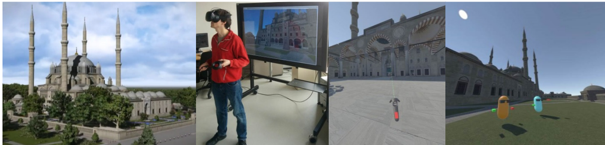
Fig. 4. The Selimiye mosque of Edirne (left), the VR System HTC Vive in action using the controllers for interacting in the environment (centre left), navigation controller for the motion in the environment (centre right) and the multi-user feature of the HTC Vive presenting two avatars with controllers (right).
