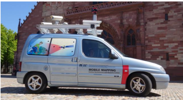
Figure 2. Our mobile mapping research platform shown in a configuration with multiple stereo camera systems and a single panoramic camera.
