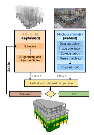
In the presented approach the 3D as-built state is calculated from photogrammetric images using multiview stereo reconstruction. Different acquisition strategies and techniques, namely (i) terrestrial acquisition with a hand-held camera, (ii) aerial acquisition using a Unmanned Aerial Vehicle (UAV) and (iii) acquisition using a fixed stereo camera pair at the boom of the crane, are tested on three test sites.
