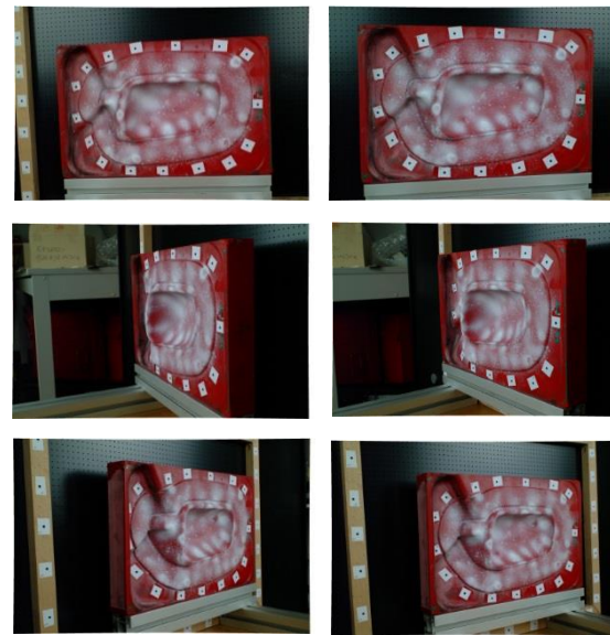
multi-image matching of car mirror forging template
