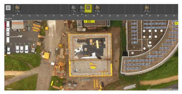
A time-series of 2D maps generated by a mosaic of multiple images. These images are orthographic: perspective-free, fully scaled, measurable and georeferenced. This time-series provides important information on the progress of the project, and can help detect scheduling problems.
