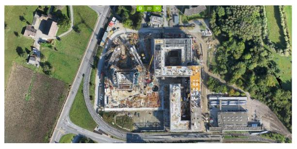
2D map generated from multiple drone-captured images. This map is orthographic, meaning perspective-free, fully scaled and measurable, and georeferenced. It is typically used to verify the as-built site status and provide up-to-date visual and survey data.
