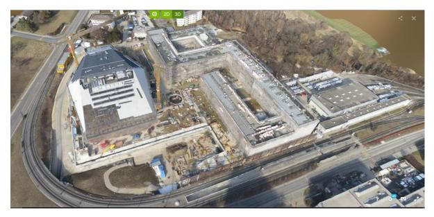
3D computer model, created from multiple drone images. This data is geometrically correct and used to compare the as-built status of the site with the design models. Custom videos of the model can be made for project review and publicity.
