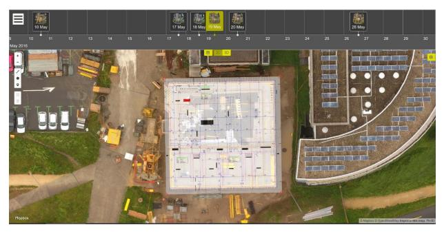
A 2D as-built map compared to the as-design drawing taken from the BIM application. This allows the as-built status of the project to be understood, and any errors spotted early. Also, the scheduling can be verified.
