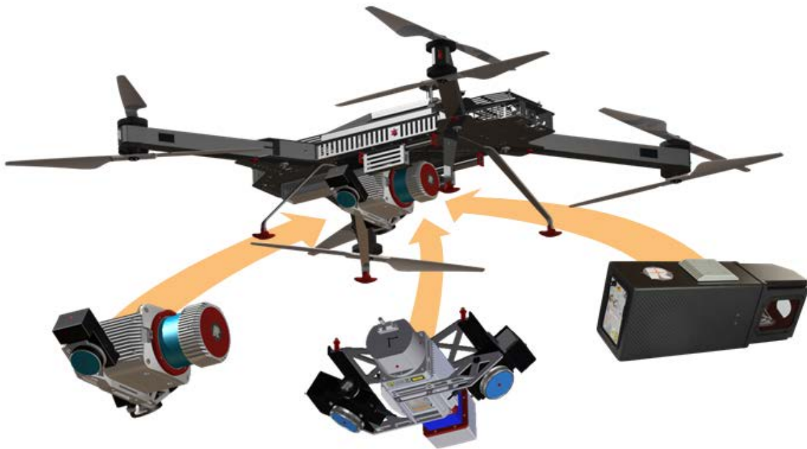
Figure 5: From left to right: RIEGL VUX-1UAV LiDAR sensor with camera option, the RIEGL miniVUX-1UAV with camera option and the bathymetric depth finder RIEGL BDF-1. The LiDAR sensors are compact and lightweight to be mounted on a UAV for data acquisition.
