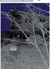
Encoding by **reflectance** (-20 dB to 3 dB, with respect to diffuse white target) Brightness independent of object distance.
