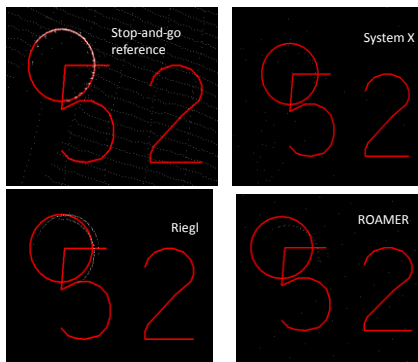
Points <50 cm above ground, top view Pole diameter 37 cm, distance to trajectory 12-15 m
