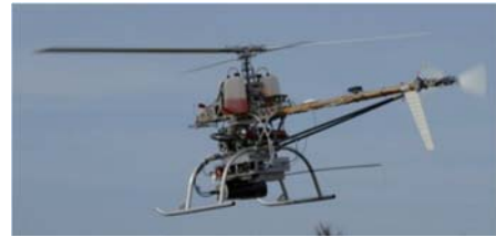
Scout B1-100, Aeroscout (Tests with Riegl Laserscanner)
