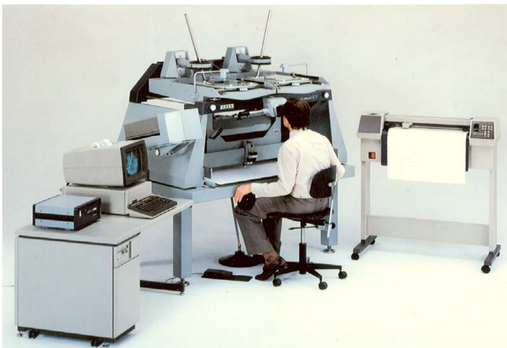
E 3 Planicart analog precision plotter connected to HP 1000 A microcomputer with HP 7580 drum plotter. Measurement supported by program package PLANIMAP/PLANI-AS and VIDEOMAP system for superimposition.
