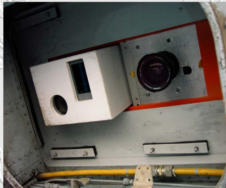
Installed in a helicopter with an Optech ALTM Lidar-System
